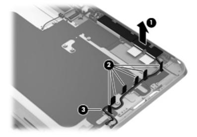
4. Remove the WLAN antenna cables and transceiver.
